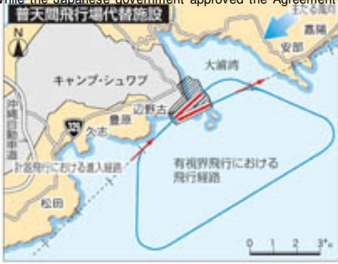
Henoko V-shaped 1,800 meter runway extending to Oura Bay
