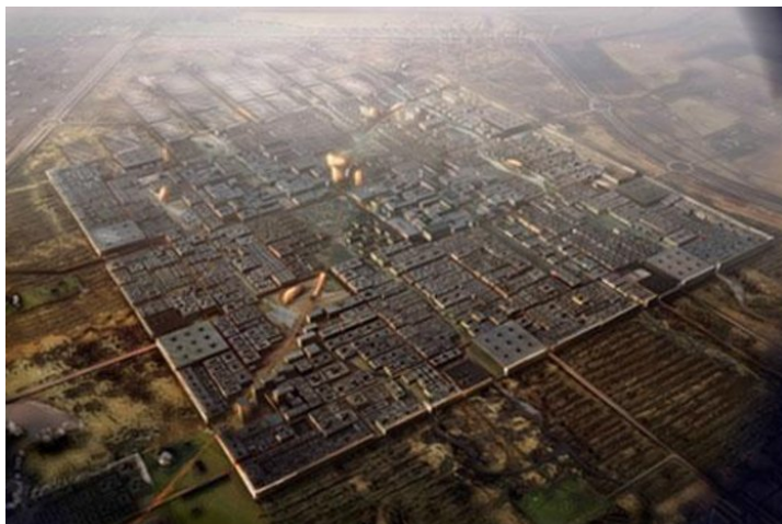
An architect's rendering of Masdar's walled city, designed with narrow and shaded streets to shut out hot desert winds
