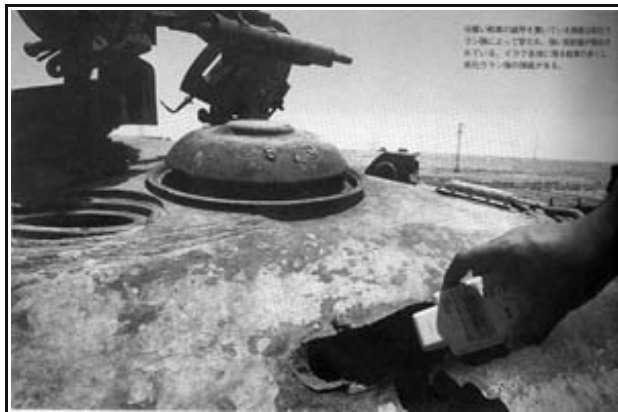
The bullet holes that pierced the armor of these tanks were caused by depleted uranium shells and strong radiation is observed.
